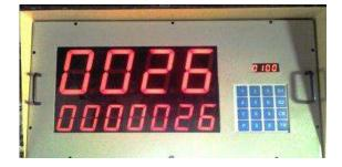
The instrument is single Microcontroller based, SWITCH MODE POWER SUPPLY UNIT (SMPS), KEYPAD for programming & counter setting & resetting, seven segment display unit for displaying running COUNT, TOTALIZER, SET/PRESET COUNT. Use of HIGHLY DURABLE SENSING HEAD instead of conventional optical sensors & proximity switches gives better results, longer life in dusty (CEMENT INDUSTRY) and rough industrial atmosphere. The unit comes with 3 display:-
